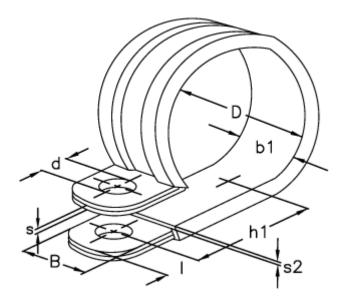
$\begin{array}{lll} b1 & = 15.0 \\ d & = 5.3 \\ Diameter D = 20 \\ h1 & = 18.0 \\ I & = 5.0 \\ s & = 0.50 \\ s2 & = 1.2 \\ Width B & = 12 \\ \end{array}$
